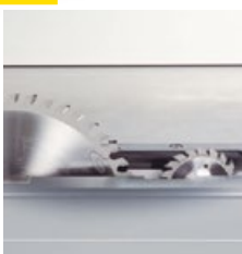
An electrical scoring unit is standard
