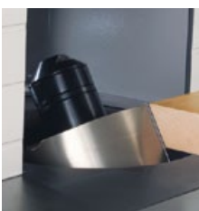
Spindle moulder tiltable from 90°–45°
