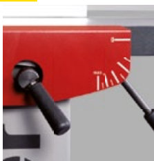
Depth of cut adjustment when planing
