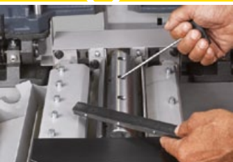
Planer knife change in seconds without adjustments
