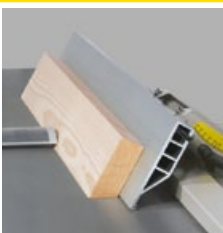
The planer fence for exact joining and beveling
