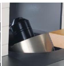
Spindle moulder tiltable from 90°–45°
