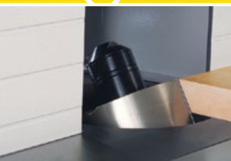
Spindle moulder tiltable from 90°–45°
