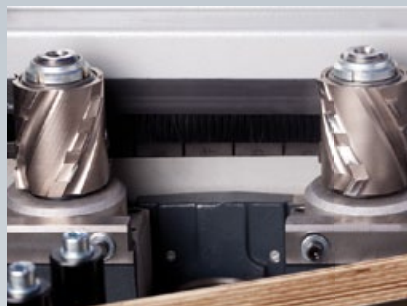
Premilling unit with diamond coated spiral cutters
