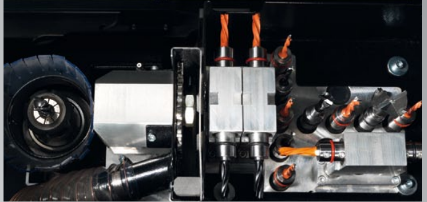
The c-express 920 is equipped with a DH14 6H 1S drilling head as standard.
