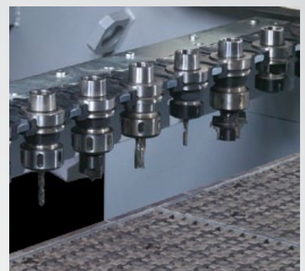
Linear tool changer allowing quick tool changes and ensuring minimum compressed air usage
