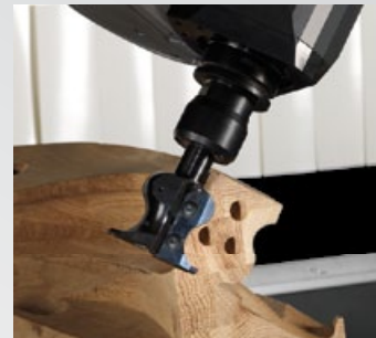
Simultaneous 5 axis processing
