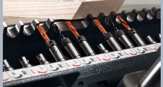
The drilling unit can be tilted from 0°–90° using compressed air.
