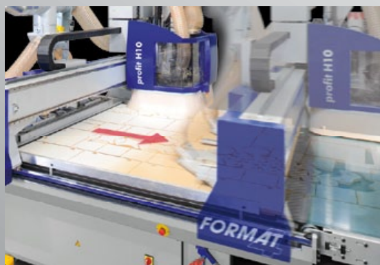
Unloading unit, removing the finished workpieces and cleaning of the table
