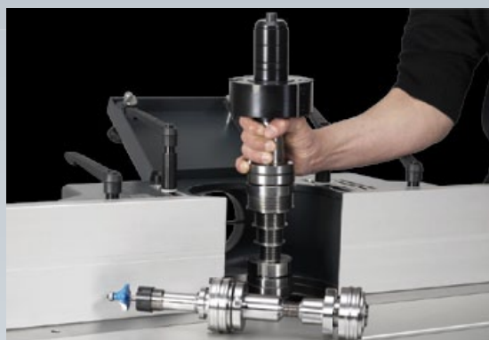
Standard: Changing of the spindle shift with minimal effort
