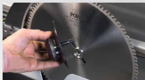
Change the saw blade without using any tools
