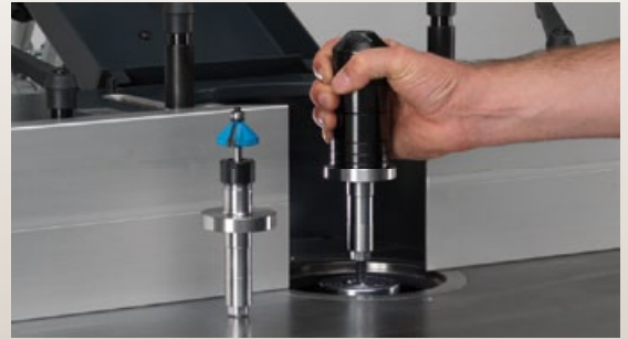
Spindle shaft quick change system: Professional level productivity for every workshop
