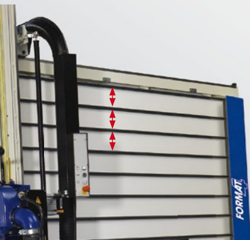
Moveable rear wall (moving spacers) When cutting horizontally the spacers move vertically to avoid being damaged by the saw blade.
