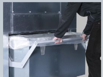
The dust collection bins are positioned under the machine ensuring an optimised, equal filling of the dust bags. The optimised clamping system ensures a quick dust bag changeover.
