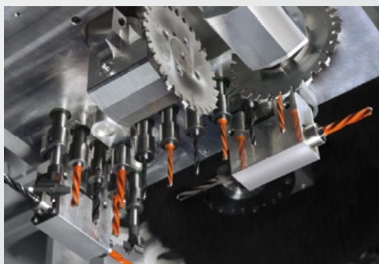
Vertical drilling spindles, grooving saws for both vertical and horizontal processing
