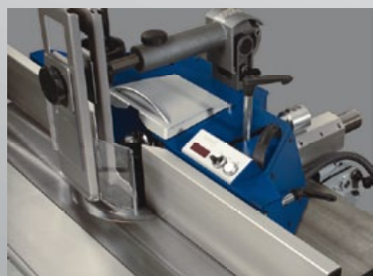
Convenient electronic spindle fence positioning
