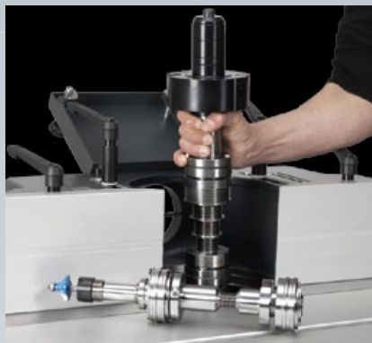
Standard: Changing of the spindle shift with minimal effort
