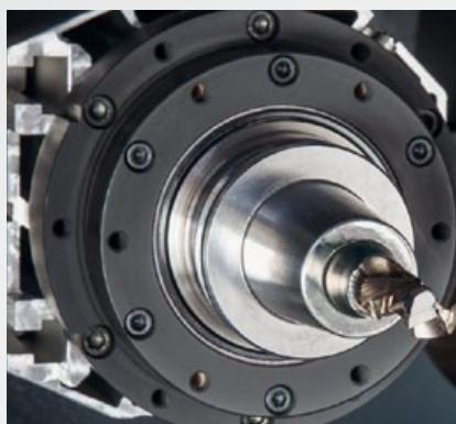
High performance main spindle with HSK-F63 collet
