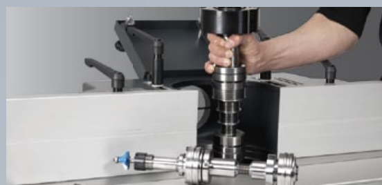
Quick spindle exchange system
