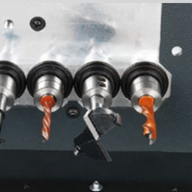
or DH 16 drilling head with 12 vertical and 4 horizontal spindles
