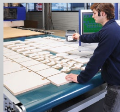
Unloading unit with conveyor belt and labelling station
