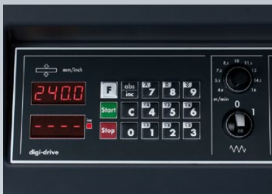
"Digi-Drive" - thicknesser table control, precision at the touch of a button
