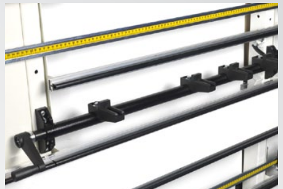
Centre support A bipartite central support designed for small workpieces runs along the total cutting length and can be easily swung out of the way when not required.
