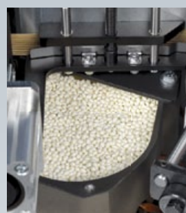
Teflon coated glue pot for hot melt granulates
