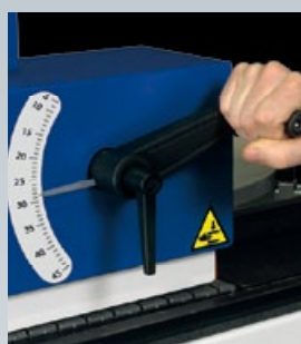
Height adjustment of the upper pressure bar
