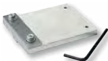
PESQW - NEW WOODWORKERS' SQUARE GUIDE The square guide raises the tool away from the tool platform. Using a set square or triangle adjust the bar to ensure a perfectly accurate position for sharpening all your chisels and plane blades
