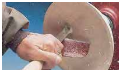
Use the curved edge for internal work
